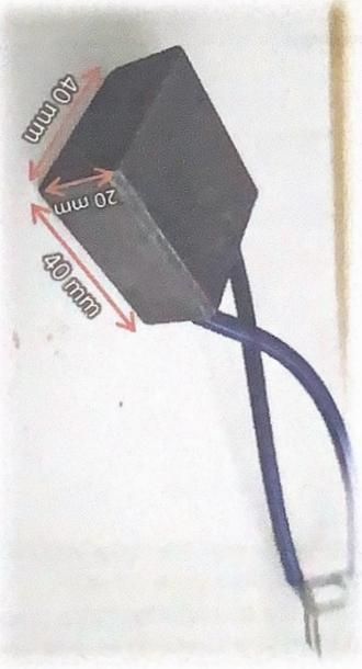
A photograph of a carbon brush. The brush is a dark, rectangular block with a blue wire attached to one end. Red arrows indicate the dimensions: 20 mm for the width, 40 mm for the length, and 40 mm for the height. |
